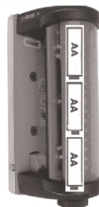
The receiver uses 3 AA alkaline batteries. Unscrew black cap at bottom of unit to replace batteries; orient as shown. Operating time is approximately 130 hours.
