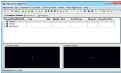
Auto Alignment tool aligns point clouds together and creates and opens a registration automatically for fast and simple registration completion.
