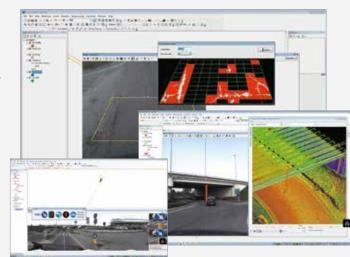
Clearance analysis, road signs extraction, pavement crack indexing and bill board extraction
