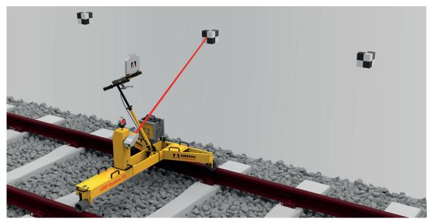
High-performance system solution for track alignment data or control-point-based tamping survey
